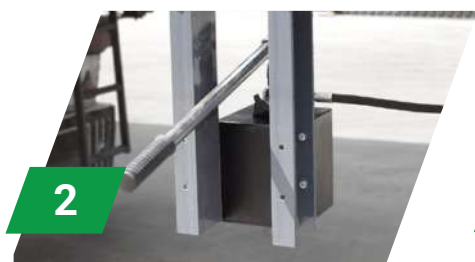
Italian pump with a handle, oil tank
